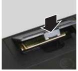
3 Your wireless keyboard is synced with your computer at the factory. However, if the keyboard does not work after installing new batteries, re-sync the keyboard with the computer by following the instructions in "Syncing the keyboard and mouse" on page 22.
